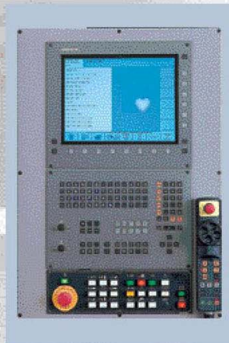
HEIDENHAIN iTNC530 Control
